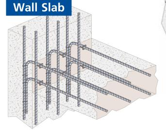
LENTON FORM SAVERS for wall/slab or wall/beam connections eliminate the need to penetrate the formwork. Indispensible when using sliding or climbing formwork.
