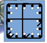
Lap splice – additional rebar in the lap zone.
